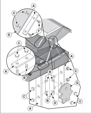
Figure 1. One Piece Breath Guard Installation
