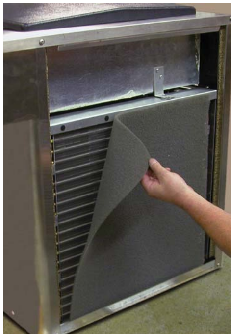
Figure 3-8 F112 Condenser Filter Removal
