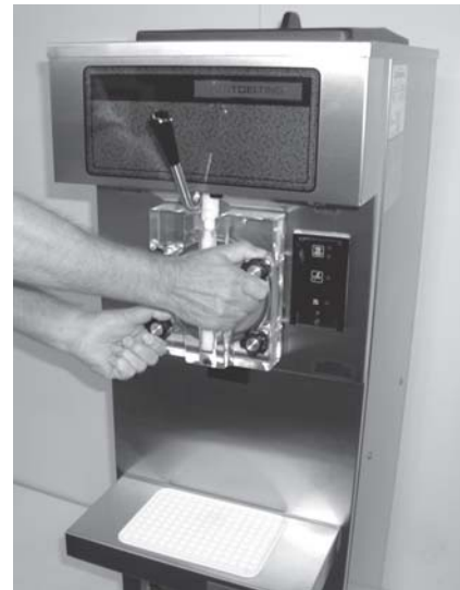
Figure 17. Removing Front Door
