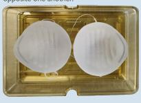
**Step 4** Place the SteamPro Lid on upside-down to allow sufficient space for the FFRs.
