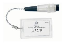
The TX27L Thermometer Test Cap (+32°F) with 6-pin Lumberg type connection.
