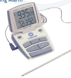
For HACCP compliance in cooking and cooling, just set the alarm. It will sound when the desired temperature is reached. Alarm can be set for temperature or time. Switchable from °F to °C. Comes with adjustable back, magnet and AAA battery. You can close the oven or refrigerator door on the 36" stainless steel, heat-resistant probe. Replacement probe: ATT865.
