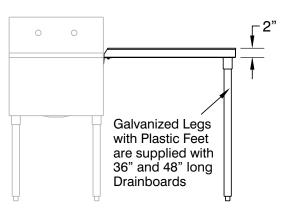
\*Drainboards 36" and 48" are supplied with legs for support.
