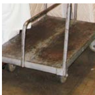
Metal—dents and rusts
