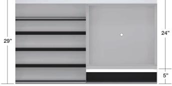
Adding a single speed rail to a **KR24** unit will increase the depth 5" to match a **KR29** unit.
