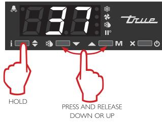
While still holding, press and release the down or up arrow to change the setting.
