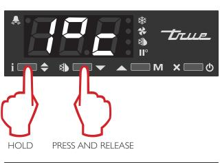
If "'F", while still holding, press and release down arrow to change to "I  $^{\circ}$  C".
