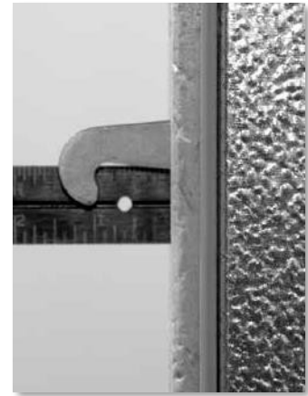
Fully Extended Cam Lock
