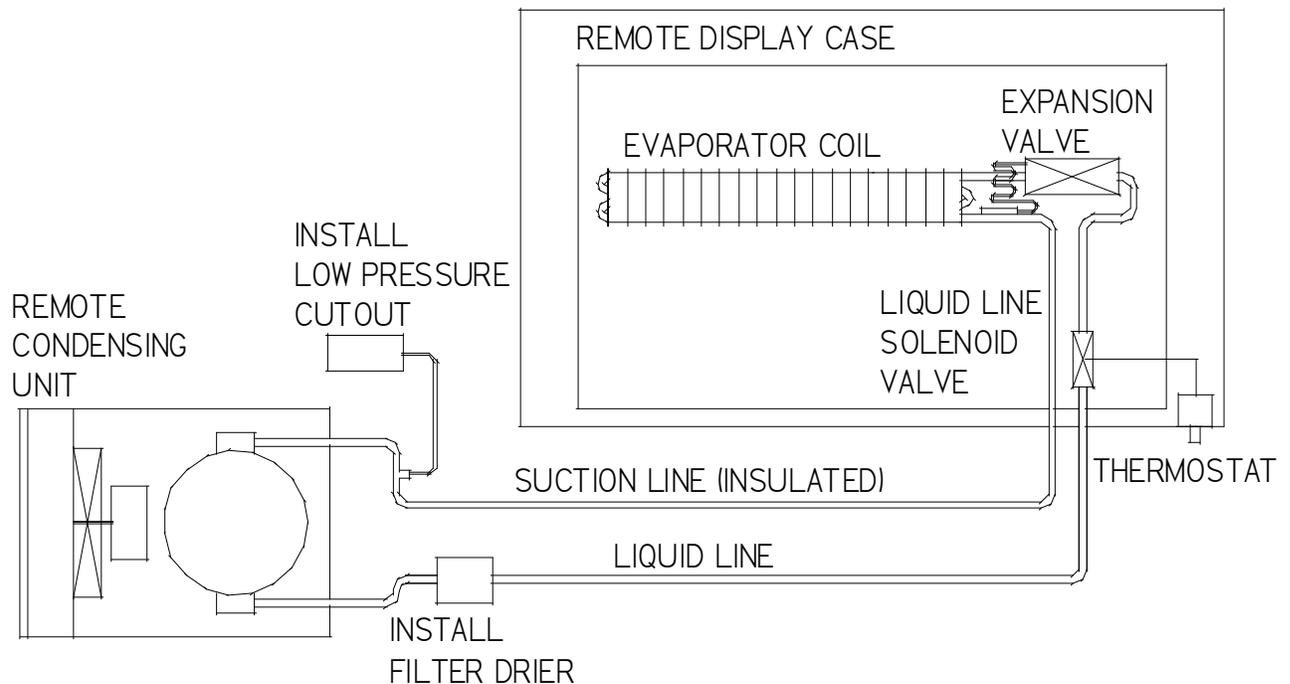
1. Mount condensing unit indoors as close to the remote display case as practical. The refrigeration line should be as short as possible.
