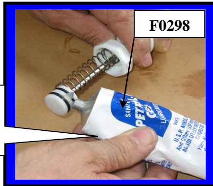
Lubricating O-rings with Petro-Gel
