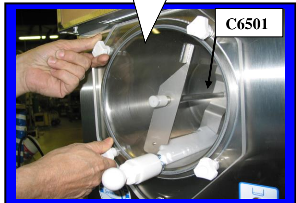
Installing large Faceplate onto front of Machine.
