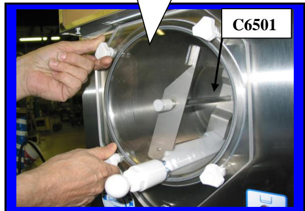
Installing large Faceplate onto front of Machine.
