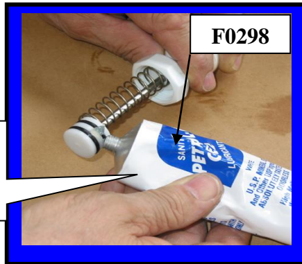
Lubricating O-rings with Petro-Gel
