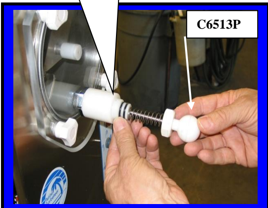
Installing Plunger Assembly into Faucet body
