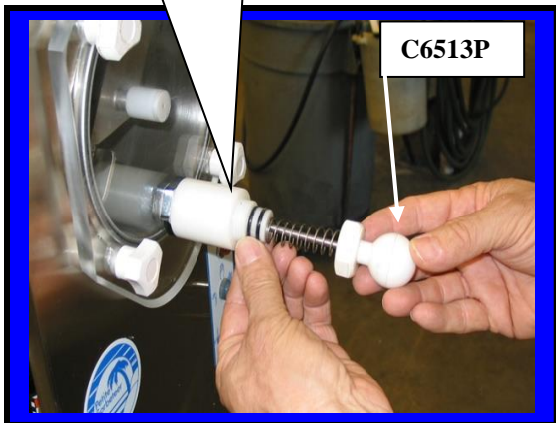
Installing Plunger Assembly into Faucet body
