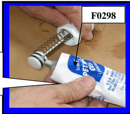
Lubricating O-rings with Petro-Gel
