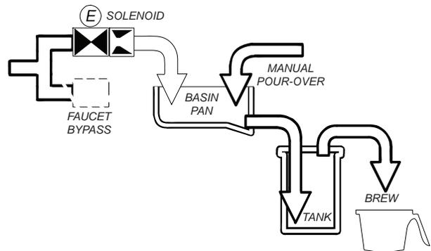
The solenoid uses a flow control device so that flow is consistent between 20 p.s.i. and 90 p.s.i.
