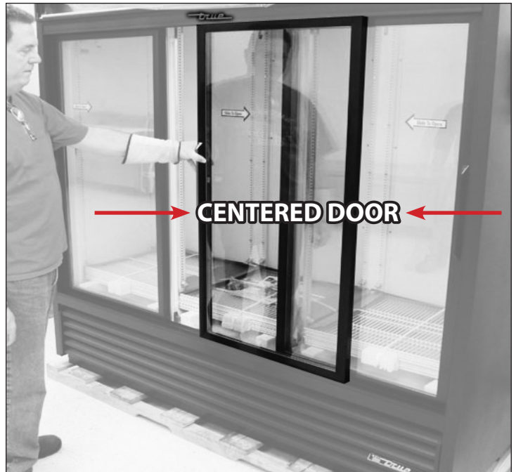
Fig. 3. Three-Door Units: Center the middle door on the left edge of the right door.
