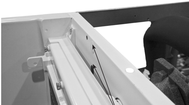
Remove Plastic Caps From Bulkhead In The Evaporator And Compressor Compartment
