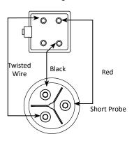
Ohm Water Level Probe and Wiring Harness
