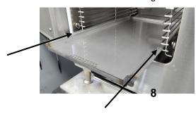
Figure 3-10 Bypass Shield Installation
