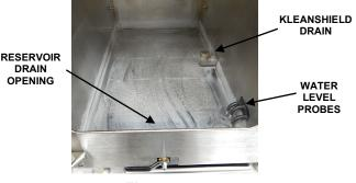
Figure 3-4 **Inspecting Compartment** (Model 22CCT6 Shown)
