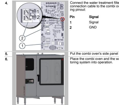
Connect the water treatment filter monitoring system's connection cable to the combi oven, observing the following pinout:
