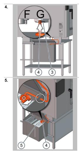
Slip the red suction tube (4) for ConvoClean forte or ConvoClean new cleaning agent onto the barbed nipple on the front bulkhead fitting (G) and secure the tube using the wire hose clamp (3) (see 'Cleaning-agent connection' adhesive label on the left unit side).
