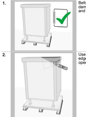
Before signing off on the delivery receipt, check the unit for damage. Document any damage on the delivery receipt and notify the carrier and manufacturer.
