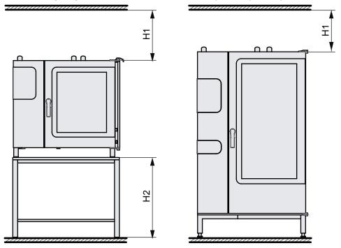
The service technician responsible for setting up the unit must take into account the ceiling's properties and any adjacent systems being used (air ventilation system, range hood) when determining the actual clearance required between the top of the unit and the ceiling. Vertical clearance H1 is only meant to serve as a reference point for the minimum vertical clearance.
