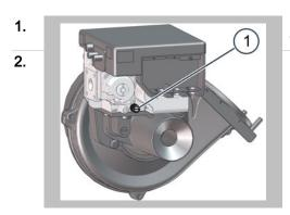
Measure the supply flow pressure at the gas valve (1) on the forced air burner.
