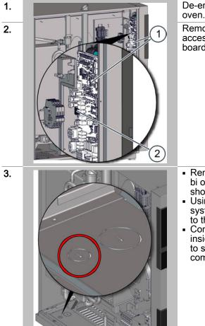
De-energize the energy optimizing system and the combi oven.
