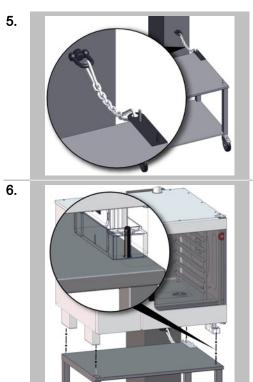
Now attach the retaining element (a chain in the figure to the left) that will limit how much the stand with casters can move.
