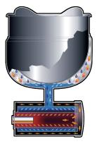
Cleveland steam jacketed kettles offer ultra efficient heat transfer, uniform heating and superior product handling. Steam jacketed kettles offer faster cooking times because two thirds of the cooking surface comes into contact with the product at a much lower temperature, compared to stock pots that use a much higher temperature
