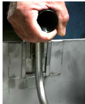
Carefully remove the filter leaf assembly.
