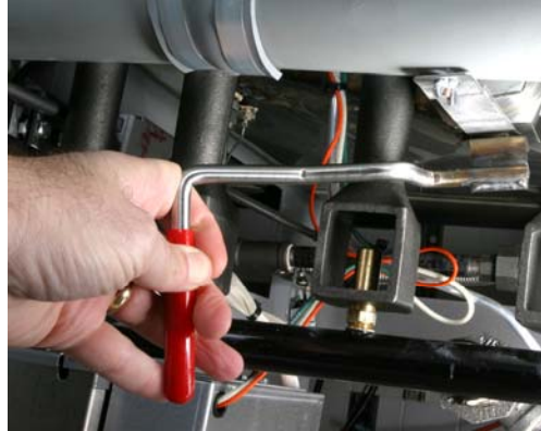
Moving the red drain valve handle to open the drain valve, allowing hot oil to drain into the filter pan.
