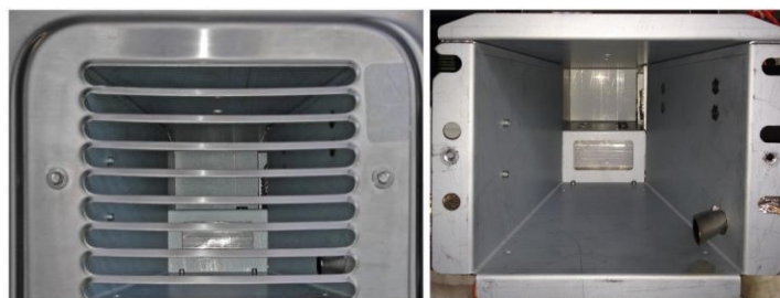
The outlet of the cooling duct carries heat to the back of the oven and is covered by a grille. The outlet comprises a sheet metal frame containing holes corresponding to the positions of Pozidriv screws securing the cooling duct to the magnetron. Use these holes for guiding the Pozidriv screwdriver.
