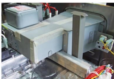
The cooling duct covers one side of the magnetron where the magnetron is attached to the cavity roof with two screws. The image shows a single magnetron 1000W e2s variant.
