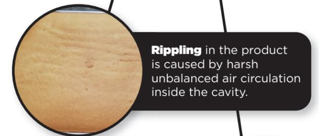
**Rippling** in the product is caused by harsh unbalanced air circulation inside the cavity.
