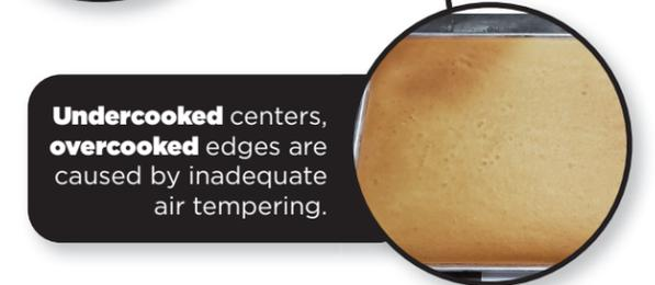
**Undercooked centers, overcooked edges** are caused by inadequate air tempering.
