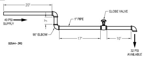
Total of above = 20 + 2.2 + 3 + 2.2 + 17 + 23 + 10 + 2.2 = 79.6 feet. Since each 10 feet is equivalent to 1 psi pressure loss, 79.6 feet is equivalent to approximately 32 psi from an original Boiler supply of 40 psi.
