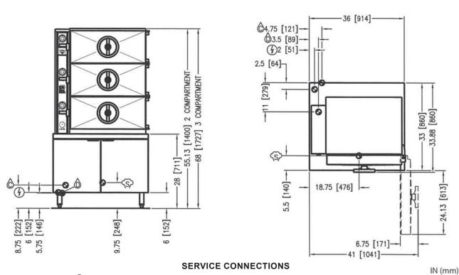
① – ELECTRICAL CONNECTION: 1/2" conduit connection to controls. 2 AMPS per compartment, 120-60-1 or 220-50-1.
