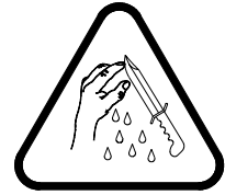
SHARP MACHINE PARTS HAZARD
