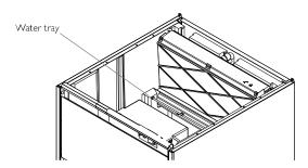
7. Switch on the machine while keeping pressed the wash button behind the front grid in order to run water pump. Let solution stand for 30-40 minutes and then switch off the machine.
