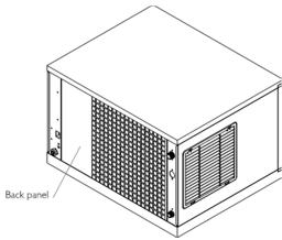
3. Clean condenser using a vacuum cleaner, soft brush or low pressure air. Clean from top to bottom, not side to side. Be careful not to bend the condenser fins.
