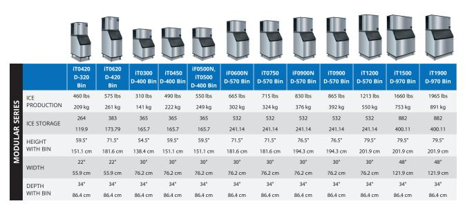
Half dice pounds produced per day. Approximate ice-making capacity based on air-cooled condenser unit at 70°F/21°C air and 50°F/10°C water. Ice machine and bin ordered separately Ice Storage is base on application capacity based on 90% of the volume x 33/lbs. /ft3 average density of ice. (iT0300 replaces iF0300 in March 2020).
