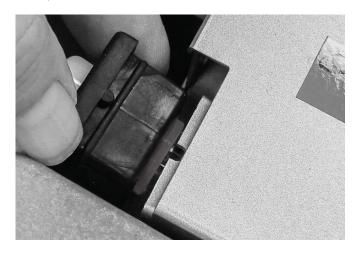
Insert bulb until it seats in the retainer stop on the opposite end.
