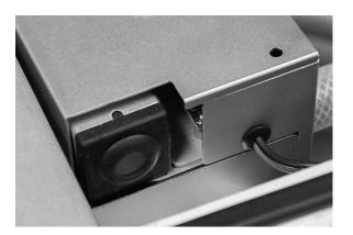
7. Attach connector to bulb.
