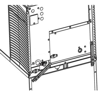
5. Secure brackets to ice machine and bin/dispenser with sheet metal screws.
