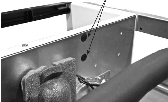
Remove Plastic Caps From Bulkhead In The Evaporator And Compressor Compartment
