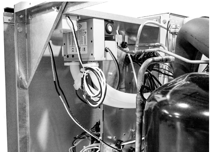
Mount LuminIce® And Power Supply To Bracket Indigo® Models Only
