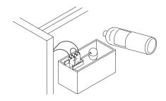
**Step 7** Move the toggle switch to the ON position. The ice machine will make ice with the cleaning solution and deposit the ice in the bin. Add the remaining cleaner/water solution as the water level in the reservoir drops.
