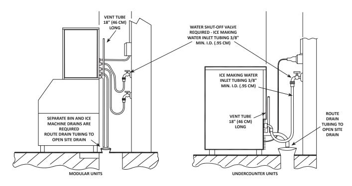
**Typical Water Supply Drain Installation**
