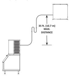
**35 feet (10.7 m) Rise:** The maximum distance the remote condensing unit can be above the ice machine.
