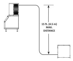
**15 feet (4.5 m) Drop:** The maximum distance the remote condensing unit can be below the ice machine.
