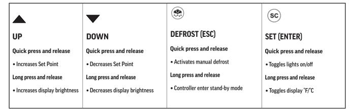
Note: When the controller is in a Standby Mode, a blue dot will be displayed as shown here. To switch out of Standby Mode, push and hold the Defrost button until the display reads ON.
