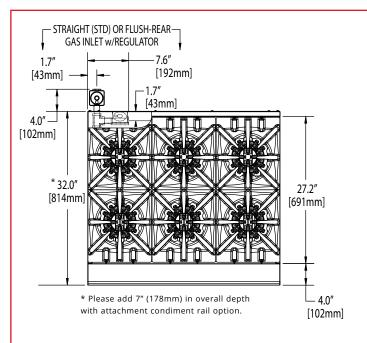
For use with Natural or Propane gas only. Gas input ratings shown for installations up to 2000 ft., (610m), above sea level. Please specify altitudes over 2000 ft. and gas type when ordering.
