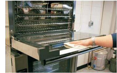
2. Clean back of outer door glass & front of inner door glass.*
