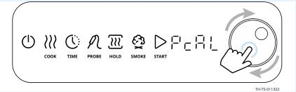
4. If the display does not show 32°F (0°C), **turn** the knob until the control displays 32°F (0°C).
