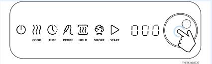
3. **Turn** the knob until the control displays PCAL.
