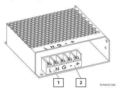
Supplies DC voltage to the control board and the ON/OFF switch.
