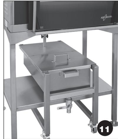
7. Turn and loosen black release knob and gently guide the telescoping funnel downward.
