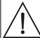
**DO NOT HANDLE NEW BULB WITH BARE HANDS. WHITE COTTON GLOVES SHOULD BE WORN WHEN REPLACING BULBS.**
