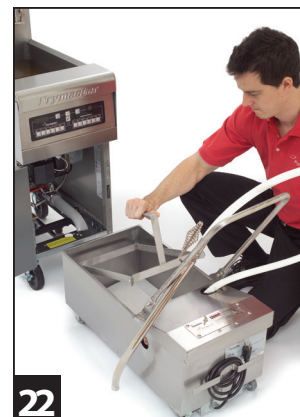
22 After filter parts have cooled to the touch, return the filter screen (making sure it is securely in place), hold-down ring, crumb tray, and lid to the filter pan.
