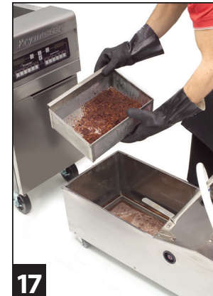
17 Remove, empty and wipe off crumb tray with paper towels. Discard crumbs into a fireproof container.
