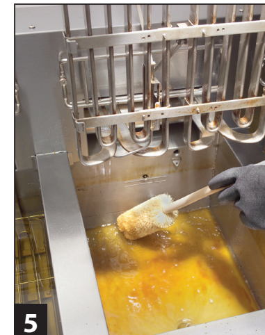
5 Brush crumbs from frypot with brush or scouring pad using circulating oil.
