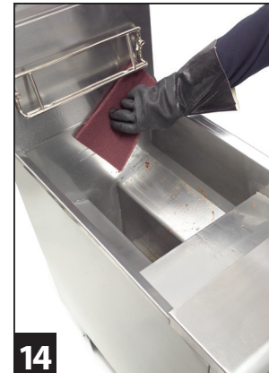
14 Use scouring pad if needed. Turn off filter pump. Then wipe out frypot with paper towels.
