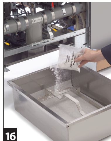
16 Sprinkle one filter powder packet (1 cup) over filter paper and return crumb tray.
