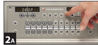
2A To count filters and utilize filtration prompts, press Filter button with controller on to start filtration.
