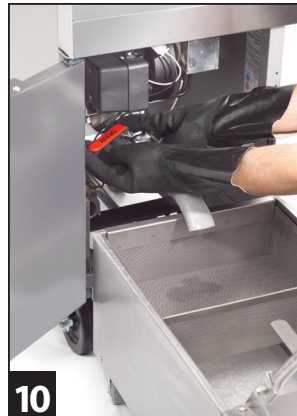
10 Open the drain valve (red handle) and allow oil to drain into the filter pan.
