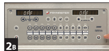
2B To bypass filter counts and filtration prompts, press OFF button to stop cooking cycle before starting filtration.
