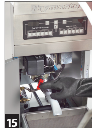
15 Close the drain valve (red handle). Hold the wand securely while turning on the filter pump. Return filtered oil to the frypot. Allow oil to bubble for 15-30 seconds to clear the wand hose of oil.
