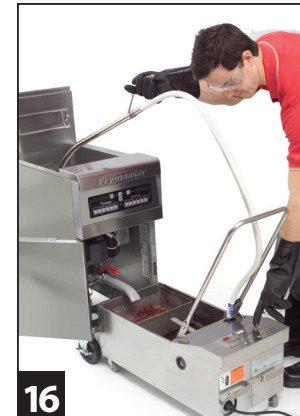
16 When all the oil is returned to the frypot, turn off the filter pump and unplug the filter power cord.
