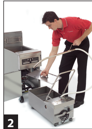
2 Retrieve stored portable filter and place near fryer. Remove filter pan lid. Make sure the filter pan is clean and prepared for filtering.
