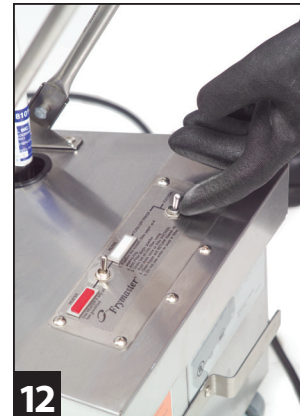
12 Hold the wand securely while turning on the filter pump. Allow the oil to circulate back to the frypot.
