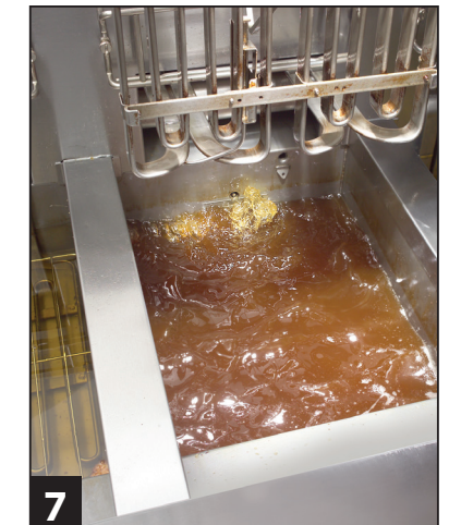
7 Close drain valve (red handle). Turn ON filter pump (yellow handle) and return filtered oil to the frypot. Allow oil to bubble for 15-30 seconds to clear return lines of oil.
