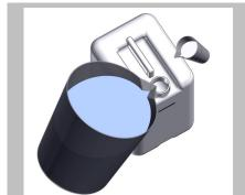
Mix the included ConvoCare K concentrate with soft water in the empty canister for ConvoCare rinse aid.
