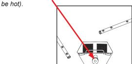
4. Remove sump strainer and pan strainer.
