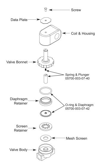
Complete 115 Volt Solenoid Valve Assembly 04810-100-53-00
