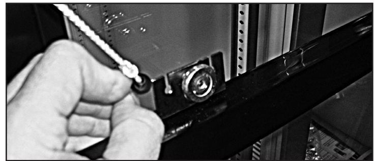
Fig. 8. Slide the black tab holding the door cord out the back
