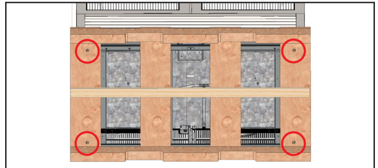
Fig. 4. Shipping bolt locations.
