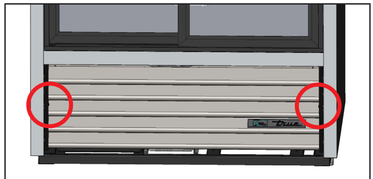
Fig. 2. Slide door louver grill screw locations.
