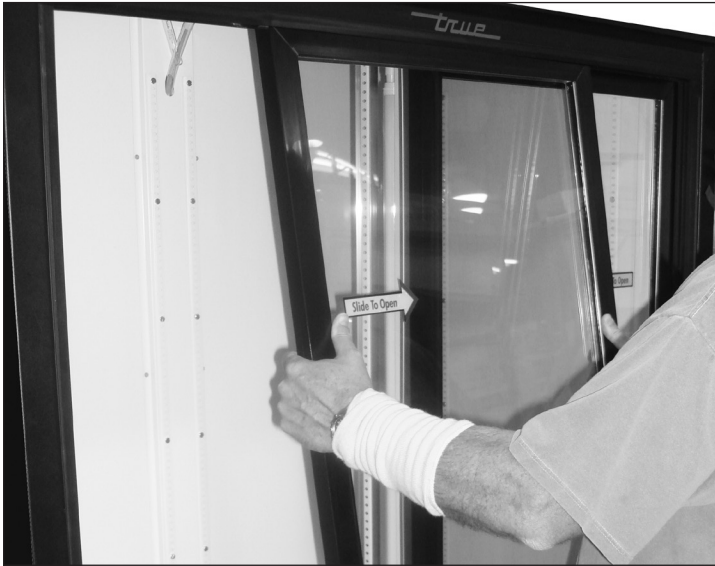
Fig. 4. Carefully remove the door.
