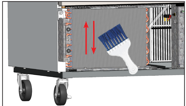
Fig. 4. Never brush across the coil fins.
