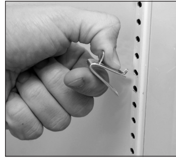
Fig. 1. Installing top tab of shelf clip.
