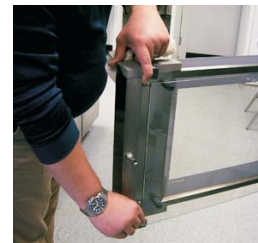
1. Open door fully. Depress glass holder clips on top & bottom of inside door, & swing open inner door glass.
