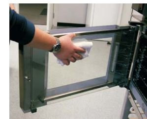
3. Swing inner door glass forward until top & bottom glass holder clips click & hold glass. Clean back of inner door glass.*
