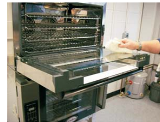
3. Clean back of inner door glass.*
