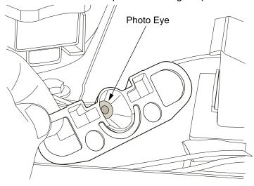
Note: Eye holders must be mounted properly. They snap into a centered position and are properly located when the wires are routed to the back and the left eye is the one with 2 wires at the connector.
