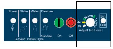
The ultrasonic ice level control allows the user to control the point that the ice machine will stop making ice before the bin or dispenser is full.
