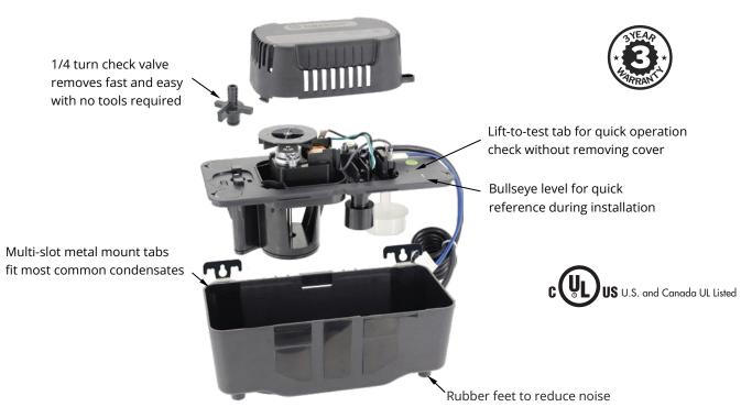
New design offers a longer 3 year warranty life and reduced noise level. Includes lid mounted bullseye level for easy installation. Rated for condensate water up to 150° F. Automatic start/stop operation with thermally protected motor.
