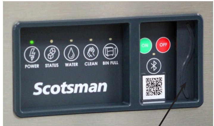
Open door to access On and Off switch buttons.
